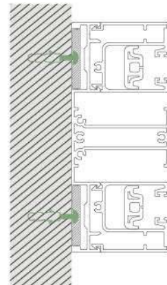
2. fissaggio cassetto a spalletta - guide indipendenti / 2. mounted cassette box in the reveal - the guides do not support it
